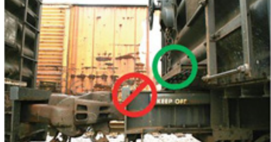
Step only on the designated walking platforms to access the handbrake
