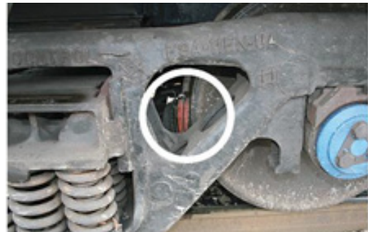
Observe that the brake shoes clasp against the wheels securely.
