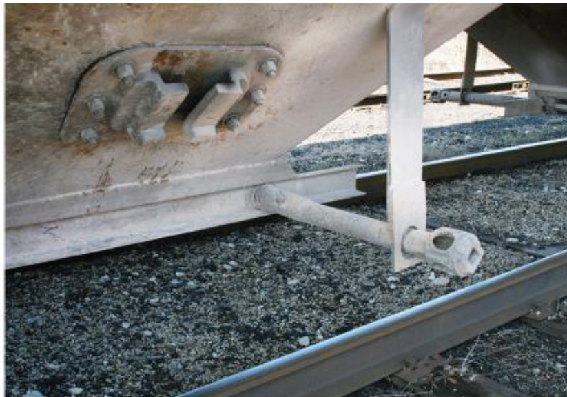
Bottom Gate doors and capstan
